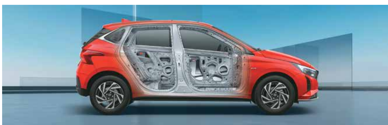
Strong body structure (with AHSS and HSS)
